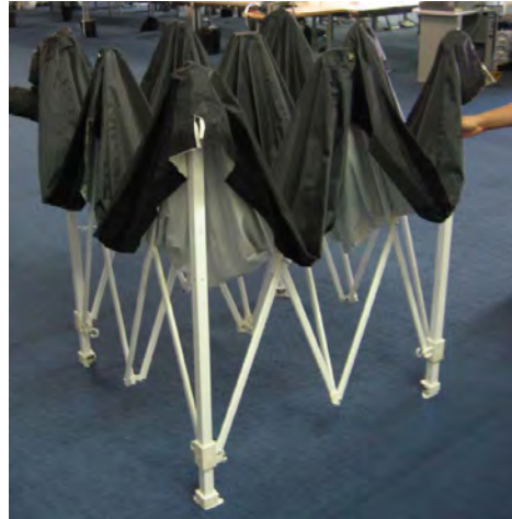
2. For quick assembly, remove the accessories and start with the frame first. The frame is easily walked into an open position with just 2 people. Pull on opposite diagonal corners to fully extend the canopy and snap it into place, then extend the legs to the top, most extended position.
